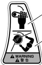
If you bend the rebar with a large angle while placing your hand onto it, there is a fear of getting your hand caught in by the fold-back reaction of the rebar.
