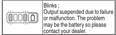
As the remaining battery indicator shows somewhat differently depending on ambient temperature and battery characteristics, read it as a reference.
